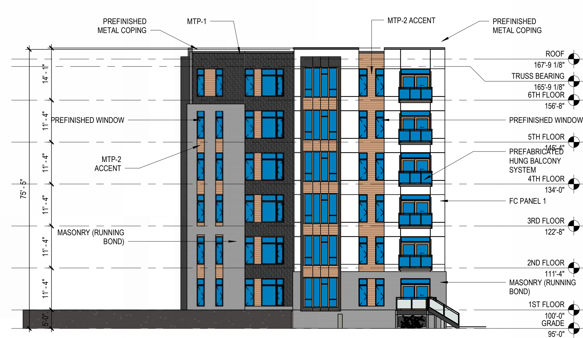
5 BUILDING B - NORTH ELEVATION 1/16" = 1'-0"
