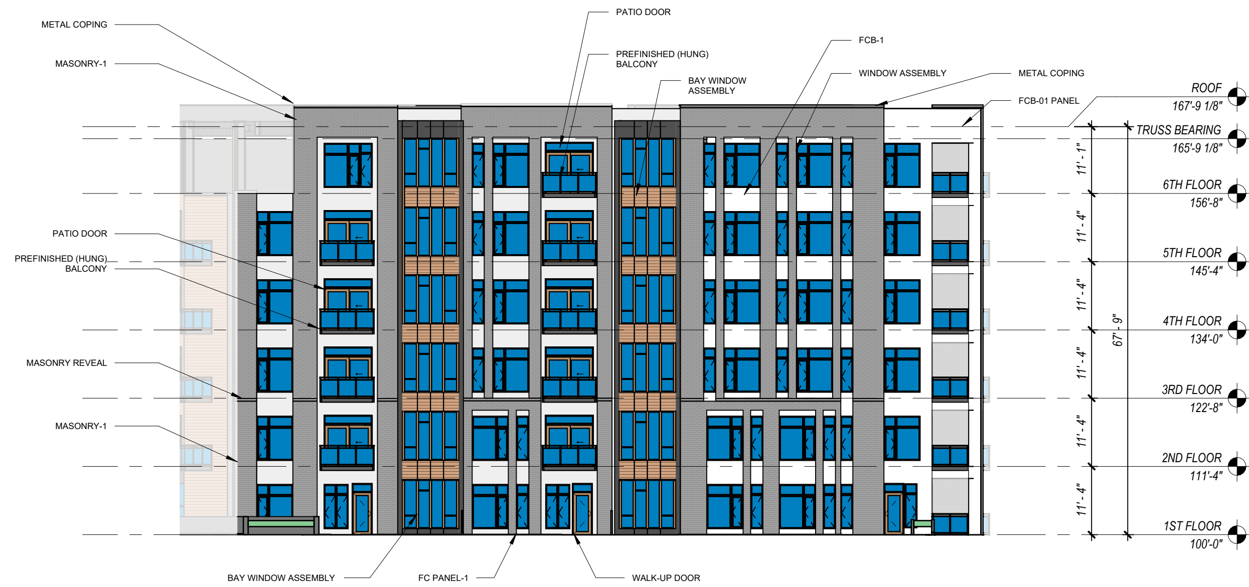
2 BUILDING A - SOUTH EAST ELEVATION 1/16" = 1'-0"
