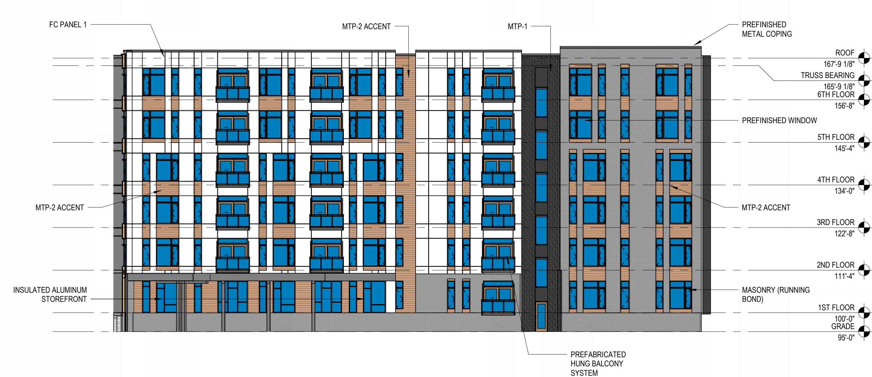
2 BUILDING B - WEST ELEVATION (S) 1/16" = 1'-0"
