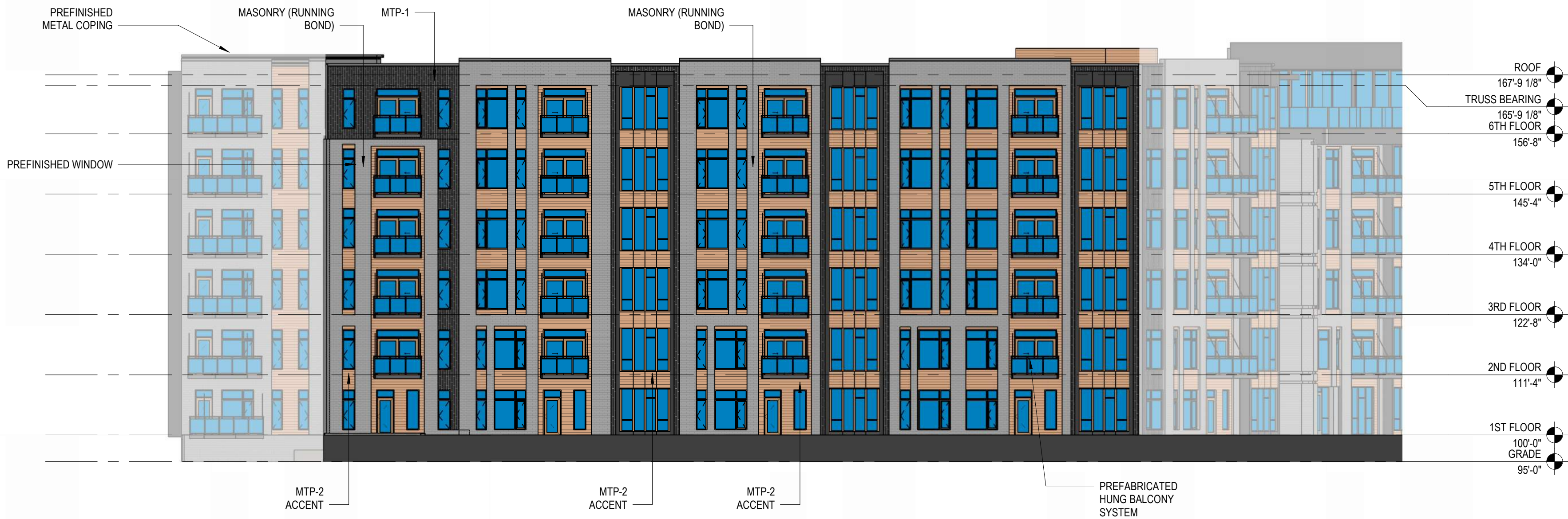
2 BUILDING B - EAST ELEVATION (S) 1/16" = 1'-0"
