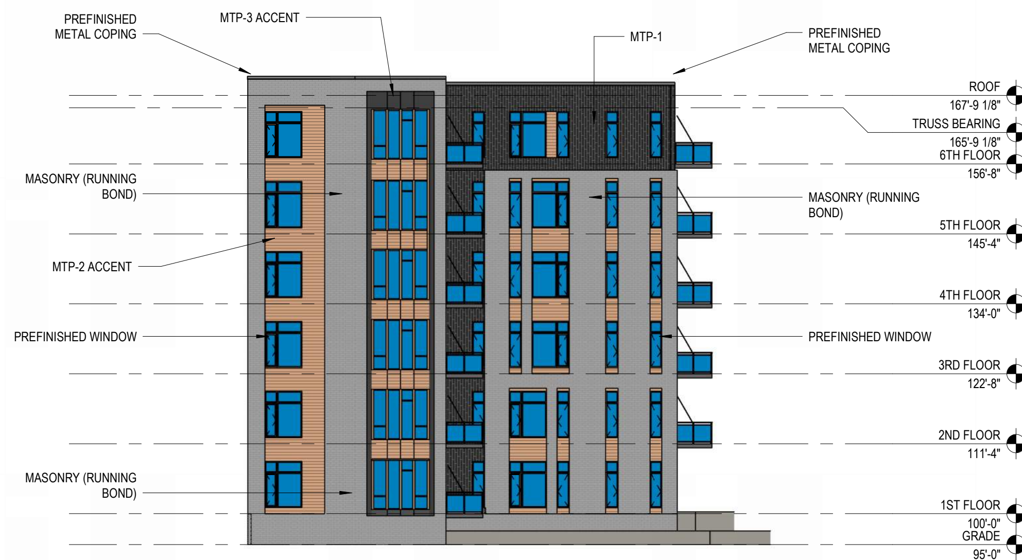
3 BUILDING B - SOUTH ELEVATION 1/16" = 1'-0"
