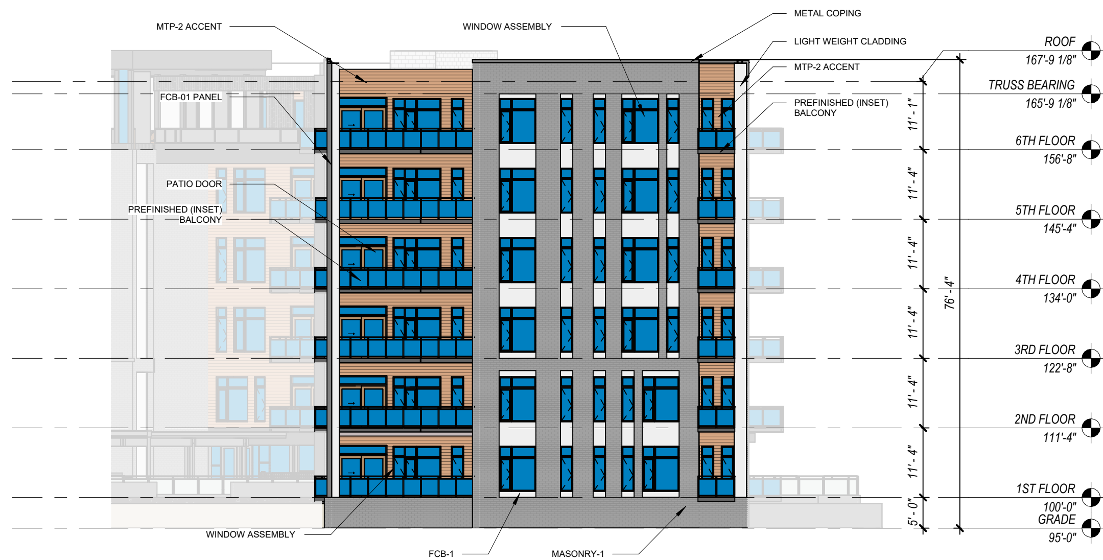
3 BUILDING A - EAST END ELEVATION 1/16" = 1'-0"
